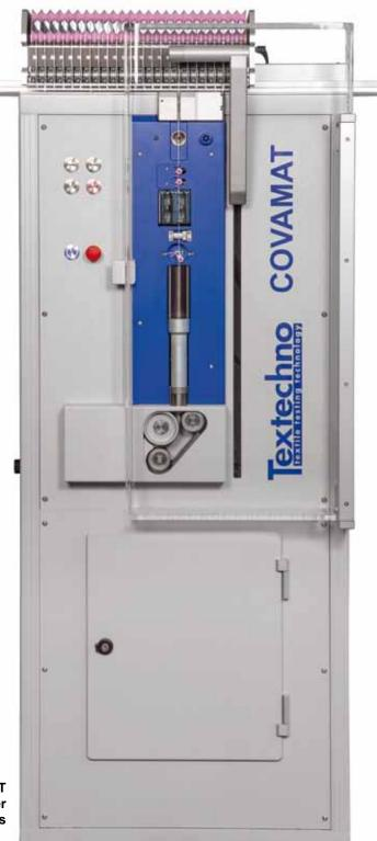
COVAMAT Automatic capacitive evenness tester for filament yarns
