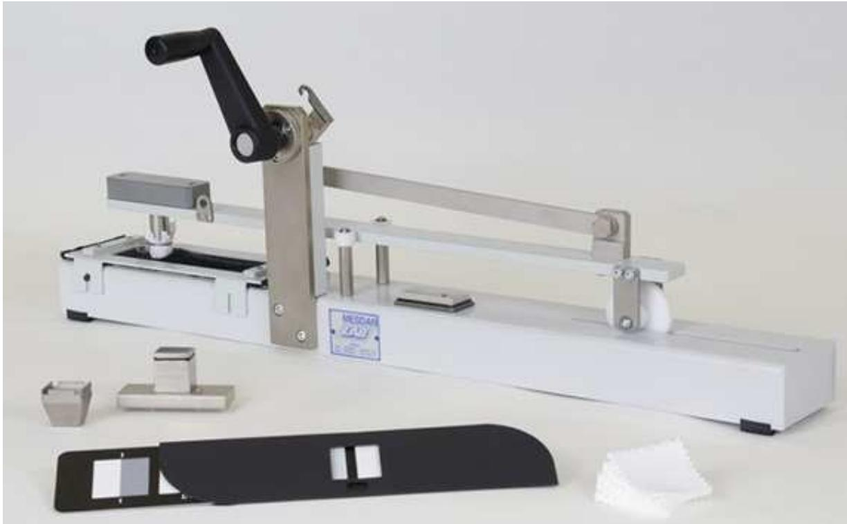
Hand driven instrument to check colour fastness on any type of textiles. It is fitted with a counter with digital reading.
