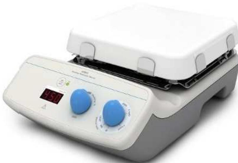
The built-in electronic system keeps the stirring speed constant, even when the viscosity of the liquid changes (counter-reaction).
