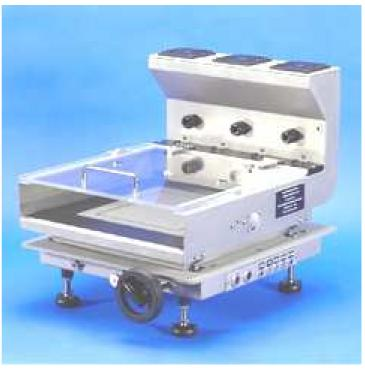
airflow hood, gravity fed fluid supply system, and ambient temperature and humidity probes. An adjustable height airflow hood easily accommodates a variety of sample thicknesses, and our ThermDAC Control and data logging system that makes testing as simple as clicking the mouse and walking away. Two hotplate sizes are available: an 8" (20.3 cm) square plate with 2" (5 cm) guard, code 3123, or a 10" (25.4 cm) square plate with 5" (12.7 cm) guard, code 3123\_.
