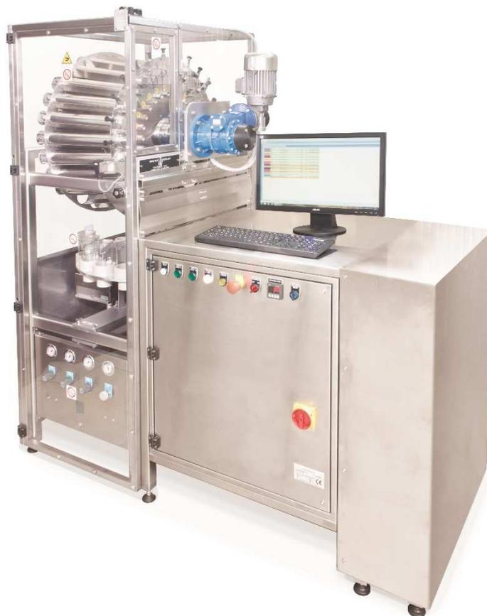
Laboratory equipment with “gravimetric” system for the automatic dosing - hence high precision and repeatability - of stock solutions, auxiliary chemicals, dilutions, and final dyeing recipes.
