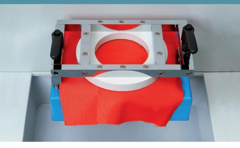
The **Water Proof** is conceived to analyse the water permeability under static and dynamic testing conditions of a wide range of textile materials. It indicates and displays the water column pressure at the moment in which the first water drops appear on the fabric's surface.
