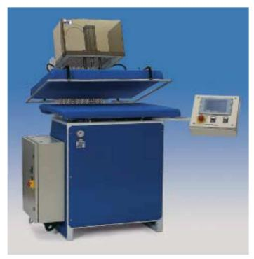
The instrument is endowed with a compressed air inlet pressure regulator, allowing to adjust the air pressure from 1 up to 6 bar.
