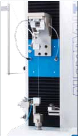
Pneumatic clamps for yarns MINI up to 20N
