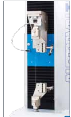
Mechanical clamps for high tenacity yarns Scott type 100-300
