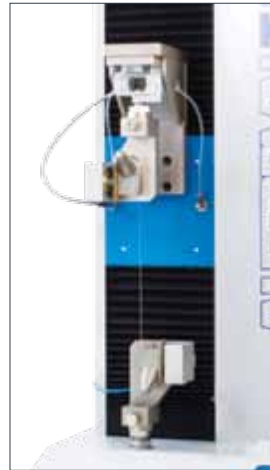
Clamps for yarns (high tenacity) with conical introducer
