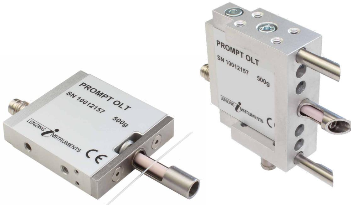
The yarn tension determines the performance of the yarn in various processes such as winding, twisting, weaving and knitting. Continuous monitoring of the yarn tension enables quick reactions to problems due to tension fluctuations, such as quench zone issues, finish tip, guide wear, winder variation, contaminated finish and human error.
