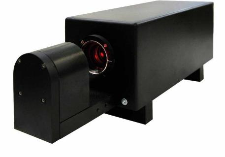
Continuous and real time information about the characteristics of produced yarn is crucial for quality control and process optimisation purposes. If feedback about defects and varying yarn properties is given not only as numerical data, but also by way of images, a thorough analysis of the momentary yarn condition can be realized.
