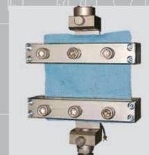
Mechanical grips for fabrics' tensile and Grab test
