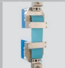
Pneumatic grips for fabrics' tensile and Grab test
