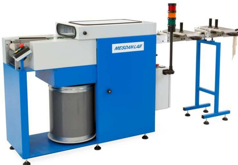
The "STIROLAB" is equipped with a swivel pot for ribbon collecting.
