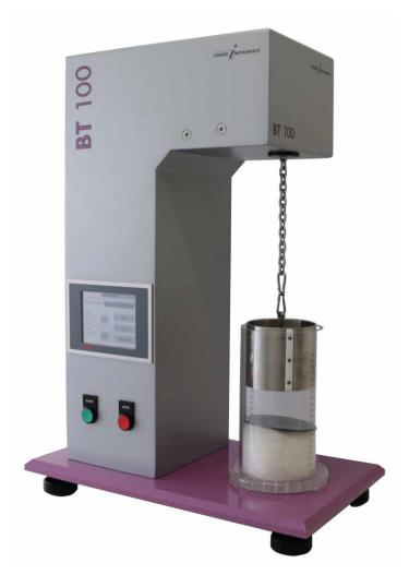
The comfort and functionality of pillows and similar end products are characterised by their firmness, capacity to retain shape and to give support. By testing filling materials like staple fibers for their compressibility, filling power and recovery properties, the requested comfort can be determined and accomplished.
