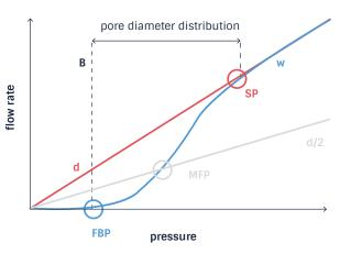
Measuring curves and resulting parameters in Capillary Flow Porometry w = wet curve d = dry curve d/2 = half-dry curve FBP = largest pore MFP = mean flow pore SP = smallest pore
