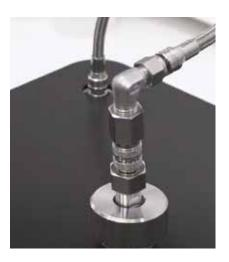
The POROLUX<sup>TM</sup> BP is a first bubble point tester, used to measure the largest pore size – often referred to as 'first bubble point (FBP)' – in media that are used for filtration and separation applications.
