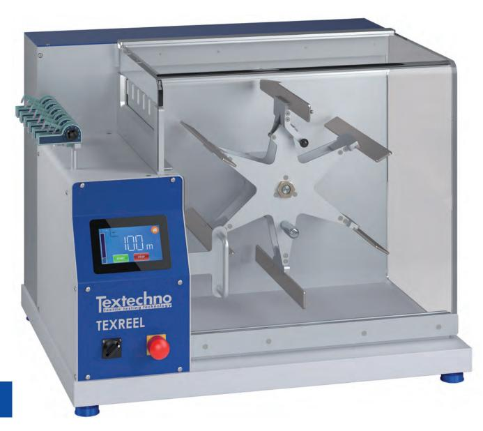
**TEXREEL** is applicable to textile yarns such as filament yarn and spun yarn. Moreover, it also works for technical yarns and reinforcement fibers used in composites such as carbon fiber tows and glass fiber rovings. Here, **TEXREEL** features a sealed housing, high torque and adjustable acceleration in combination with a tangential stripping creel that is also provided through Textechno.
