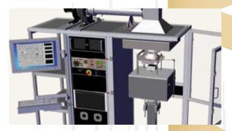
The cooling of the heat-flux meter is realized by means of a radiator and a closed cooling circuit, thus no water supply and drain is needed.
