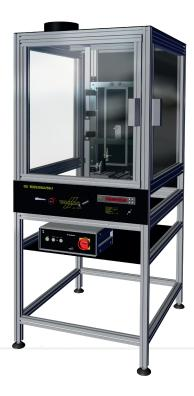
Test device, consisting of test chamber, burner and specimen holder, fine adjustment valve propane, shutoff valve propane, electronic stop watch Control unit Burner movement Specimen holder
