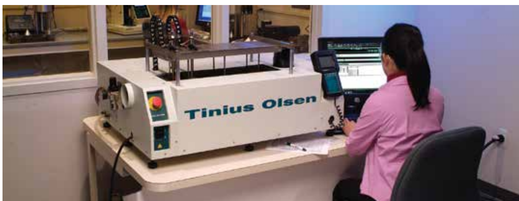
Both the Model 603 HDTM and 303 HDTM can be controlled by a PC
