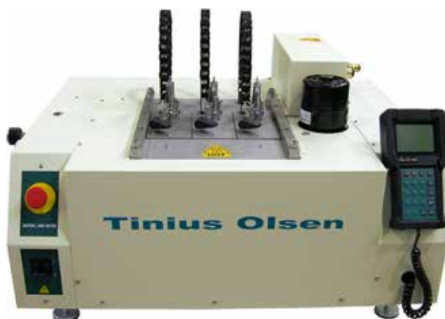
Model 603 HDTM shown with two test stations, one for deflection temperature and one for Vicat testing. The stations are raised for easy and rapid specimen insertion prior to a test and for specimen removal at the end of the test.
