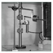
Counterbalance Support — This option is used to support the extensometer and is commonly used when the extensometer is attached to small or fragile samples.
