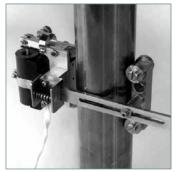
**Extension Bracket** — This option allows the extensometer to be used with samples that are thicker than maximum opening of 0.625 in/16 mm on the standard model. There are three choices with this option where an extension bracket allows the extensometer to be mounted on samples that are either 1 in/ 25 mm, 2 in/50 mm or 3 in/75 mm thick. Note that this option is only available for non-averaging extensometers.
