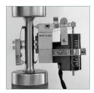
Averaging — In this type of extensometer, knife edges are placed on opposite sides of the specimen to provide an average amount of strain between the two gauge points.
