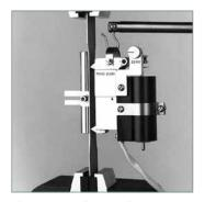
Sheet Metal Attachment — This option allows the extensometer to accommodate thin, flat specimens. Note that this option is only available for non-averaging extensometers and typically requires the use of a counterbalance to support the extensometer.
