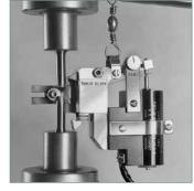
**Breakaway Release** — This option is ideally used when measuring strain on samples with brittle characteristics and which may cause premature failure. This option typically requires the use of a counterbalance to support the extensometer and is available for both averaging and non-averaging type extensometers.
