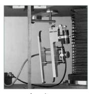
Pneumatic Release — This option is combined with a swing away support and allows the remote release of the extensometer from the sample.
