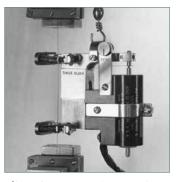
Film Clamps — These spring activated clamps allow precise strain measurement of thin materials up to 0.125 in/3 mm thick, including plastics and foils, without marring the specimen. Note that this option is only available for non-averaging extensometers and typically requires the use of a counterbalance to support the extensometer.
