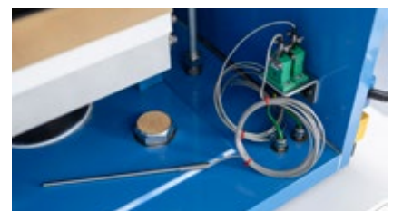
Connection for external thermocouple
